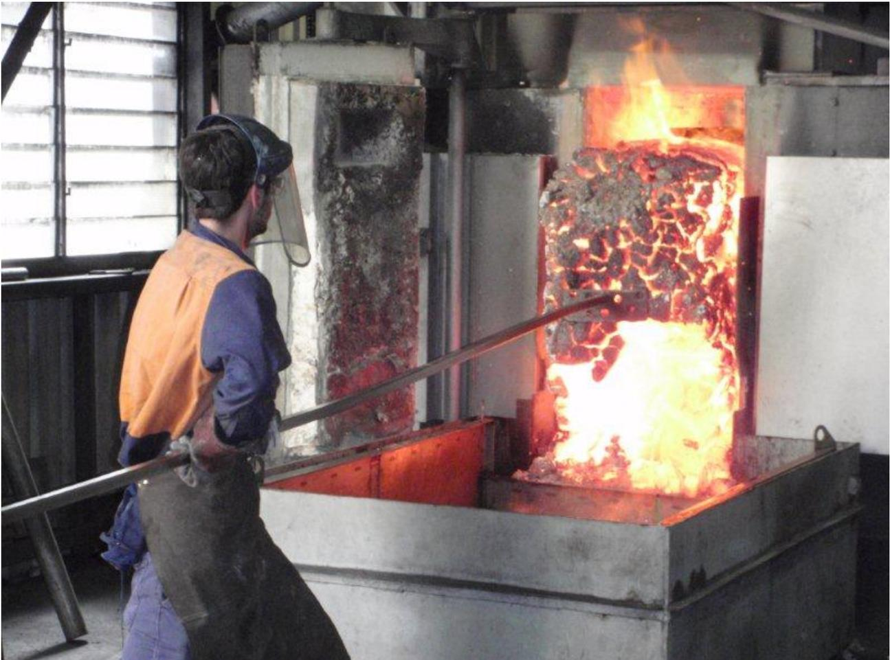
*Coke oven testing of New Lenton Coal*
